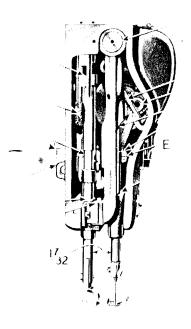
Fig. 4. End View of Machine, Showing Oiling Points
