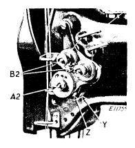
Fig. 15. Adjustment of Thread Controller
