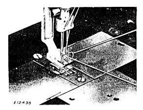
Fig. 11. Drawing Up the Bobbin Threads
