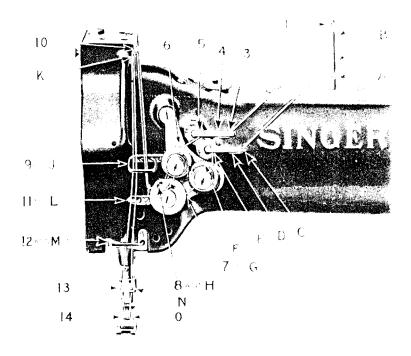
Fig. 10. Upper Threading
