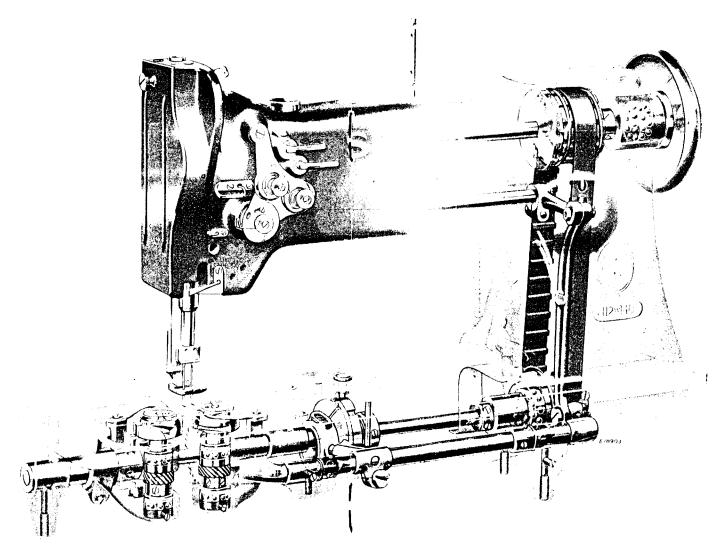
"X-Ray" View of Machine 112w140 Showing Ball Bearings and Simplified Feed Mechanism
