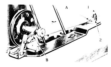
Fig. 8. Winding the Bobbin
