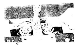
Fig. 7. Removing the Bobbins
