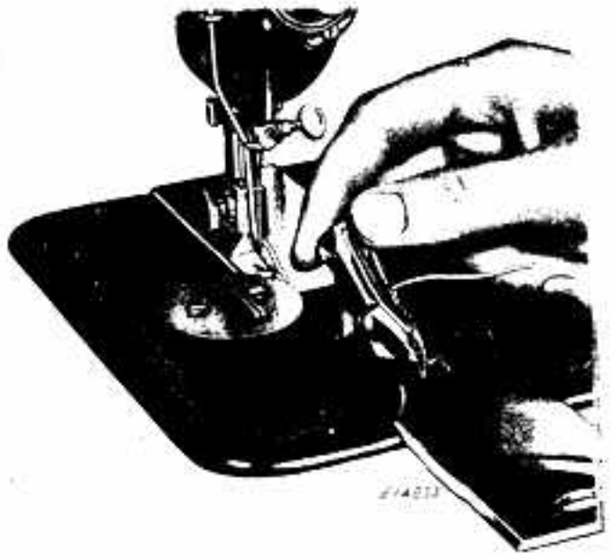
FIG. 10. REPLACING THE SHUTTLE
