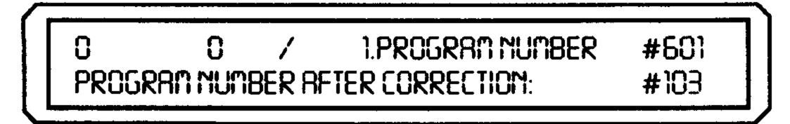
If the displayed program is to remain unchanged after carrying out the correction, a new program number must be entered for the program which is to be altered.
