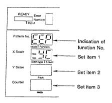
The pattern No. display gives the function No. of memory switches. Each function has as many as three different set items. The set values are shown on the X Scale, Y Scale and Counter displays. If the function does not have all of the three set items, "---" will appear on the display corresponding to the lacking set item.
