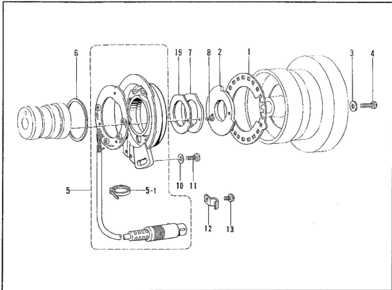
Q. 操作パネル関係/Operation panel mechanism/Schaltkasten/
